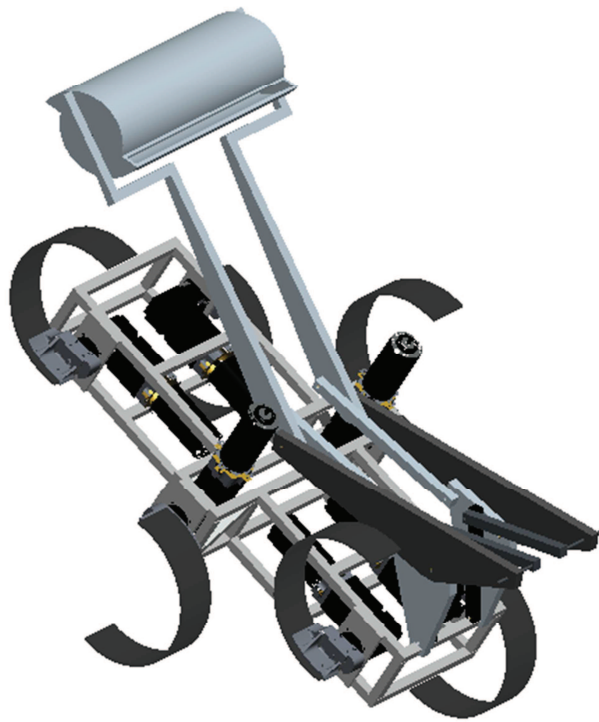
Figure 24: The excavation system located close to the center of mass for walking across the competition area.
